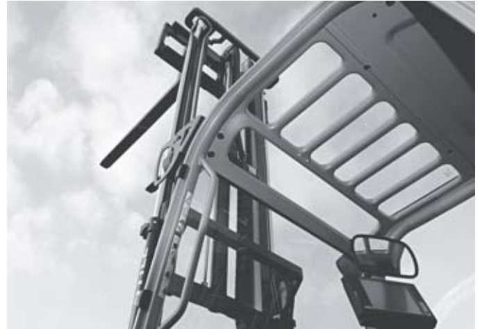
Large viewing window in the roof of the driver's cab ensures good visibility of the load above
