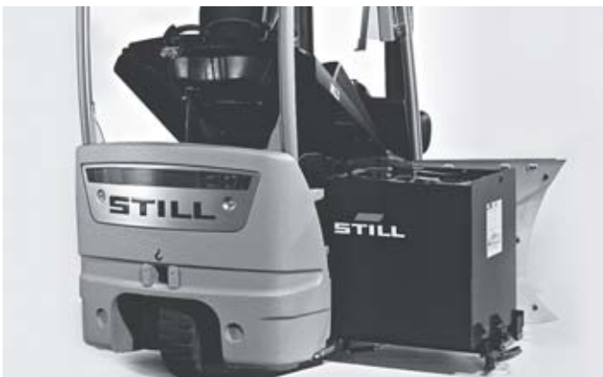
On-board battery bridge for lateral battery replacement using crane
